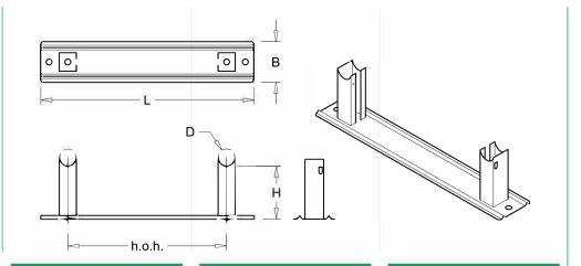
Above mentioned tube rail supports are custom made. Variables can be:
